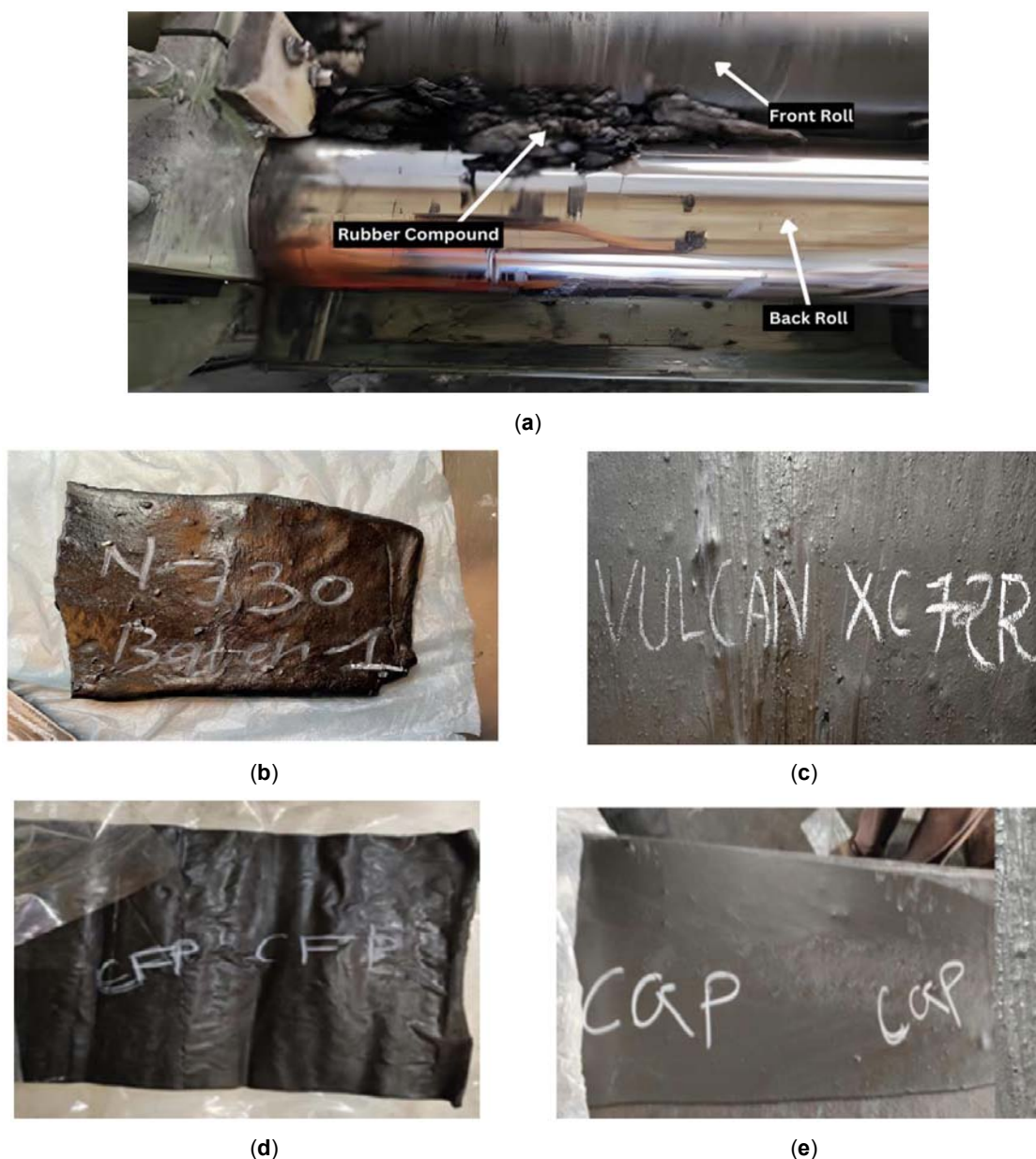
Figure 1: (a) NR/Conductive filler mixing on two roll mill (b) Sample-A NR/N-330 Composite (c) Sample-B NR/ VULCANXC72R (N-770) Composite (d) Sample-C NR/CCF Composite (e) Sample-D NR/CGP Composite.
